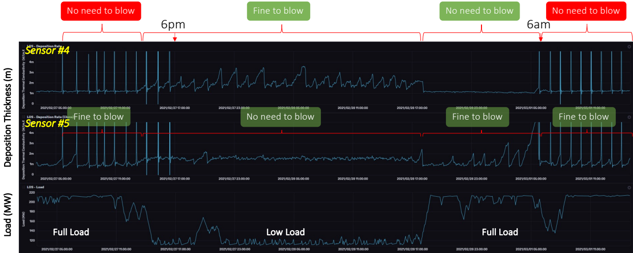
Figure 8. Deposit thickness changes between February 27 and March 1, 2021, including impacts of soot blowing.
